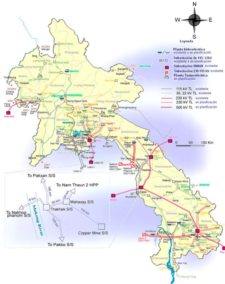
FIGURE 1: Planned Power System Diagram in 2020
